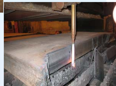
HIGH NICKEL STEEL CLEAN CUT WITH SQUARE CORNERS NO ROLL-OVER AND SLAG FREE CUTS
