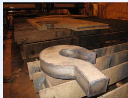
INCREASED SPEED FROM 4 IPM TO 6.5 IPM ON 8" PLATE COLD CUTTING
