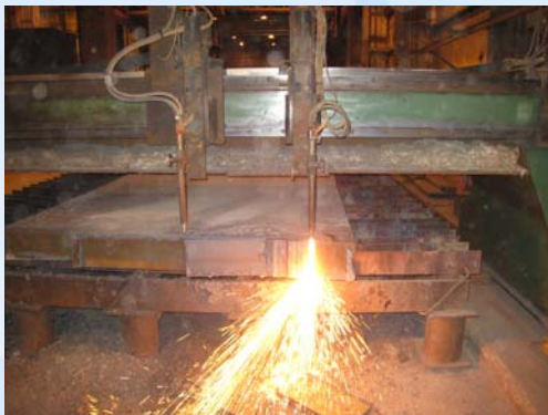
NEW OFSHX-6 PROPYLENE TIP, NO PREHEAT REQUIRED ON HIGH NICKEL 6.5" STEEL USING PROPYLENE
