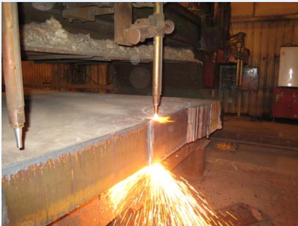
HIGH NICKEL STEEL CLEAN CUT WITH SQUARE CORNERS NO ROLL-OVER AND SLAG FREE CUTS
